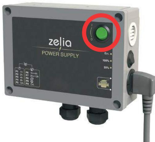
If an automatic cover dry contact is connected to the box, the switch present on the side of the box should be in EXT position to enable detection. It is still possible to flip the switch to 100% to disregard the tank cover information and force nominal production, or even to 25% to divide the production by 4 regardless of the status of the shutter.
